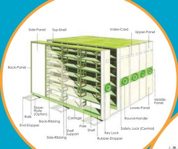
Every SquireRack Mobile Filing System is carefully designed and constructed in the highest quality, precision engineered using specially selected materials for its strength, integrity and durability. Paying attention to details, these attributes are critical considerations embraced by our R & D engineers when designing a storage system to withstand very heavy loads are concerned.
